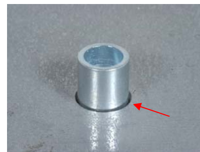
Figure 4. Large gap around self-clinching standoff indicates possibility of bell-shaped hole.
