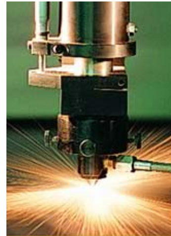
Figure 5. A high-power laser cuts a hole in sheet metal.
