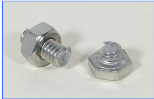
Figure 1. Galling during installation frequently leads to fastener failures such as seizing, delaminated threads and twisted heads..
