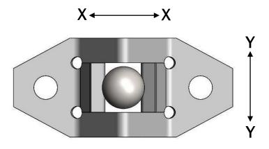
Allowable misalignment in the X-X direction is subjective and more difficult to quantify as an excessively off-center position may change the pull-out tension of the ball stud but still be acceptable. The flexibility of the ball stud clip "ears" allow for a  $\pm$ .010" standard manufacturing hole placement tolerance. Acceptability of further misalignment should be determined by testing in the application.
