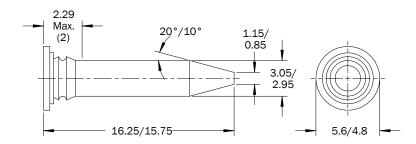
The ATCA-style pilot pin meets the ATCA PICMG 3.0 specification and features a 15° tapered point to engage easily with the mating hole. To order use part description:
