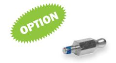
A variety of thread locking and lubricating materials can be applied to the threads. Nylon (shown), micro—encapsulated epoxy and other locking elements prevent loosening due to vibration. Lubricating coatings reduce friction, heat buildup and galling during installation of mating fasteners. To specify a nylon locking element, insert PATCH at the end of the part description. Other locking and lubricating materials available by request.
