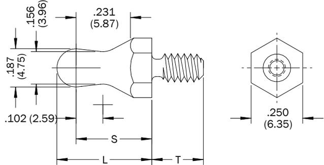
Example above for 6-32 unified thread. For M3.5 metric thread use series code BS10M.
