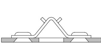
Rivet the ball stud clip onto the panel with either plain or 100° countersunk head rivets, or with screws, nuts and washers (plain rivets shown)
