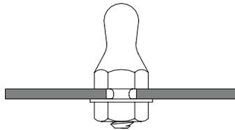
Install the ball stud onto the mating panel according to the appropriate installation method
