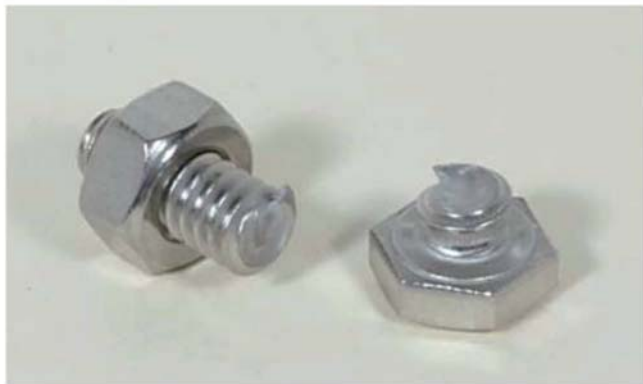
Fig. 1 — Galling during installation frequently leads to fastener failures such as seizing, delaminated threads and twisted heads.
